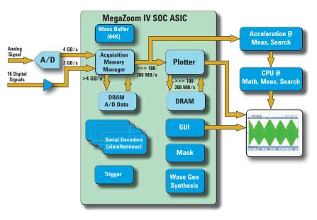
Figure 4: Agilent's MegaZoom IV ASIC combines many of the traditional discrete blocks in to a single chip that speeds the signal path considerably. In addition, it removes the oscilloscope's CPU system from the majority of operations accessing an update rate over 1 M waveforms per second.
