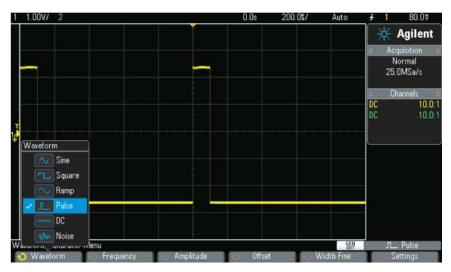
Figure 1: The integrated function generator in the Agilent 2000 and 3000 X-Series oscilloscopes uses the oscilloscope's large display to set up the waveform and saves space and money compared to a stand-alone function generator.
