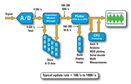
Figure 3: Traditional oscilloscope architectures use discrete components and place the CPU system in the display path of the waveform. Both of these combine to cripple update rate, often limiting it to just a few hundred waveform per second.
