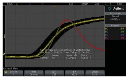
Figure 7. In this example from an Agilent 3000 X-Series scope, 2.8 million mask tests were executed in a little over 10 seconds. During this time, 85 failures were noted, resulting in a 0.0030% failure rate.
